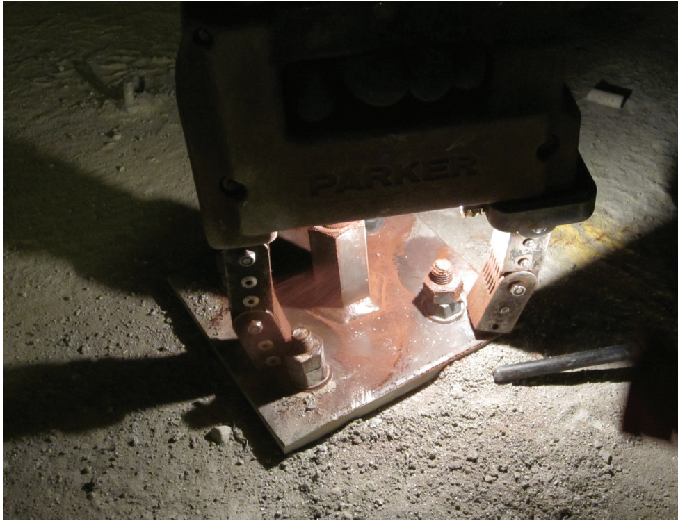
Fig. 3-7. Magnetic particle testing (photo courtesy of Simpson Gumpertz & Heger).
