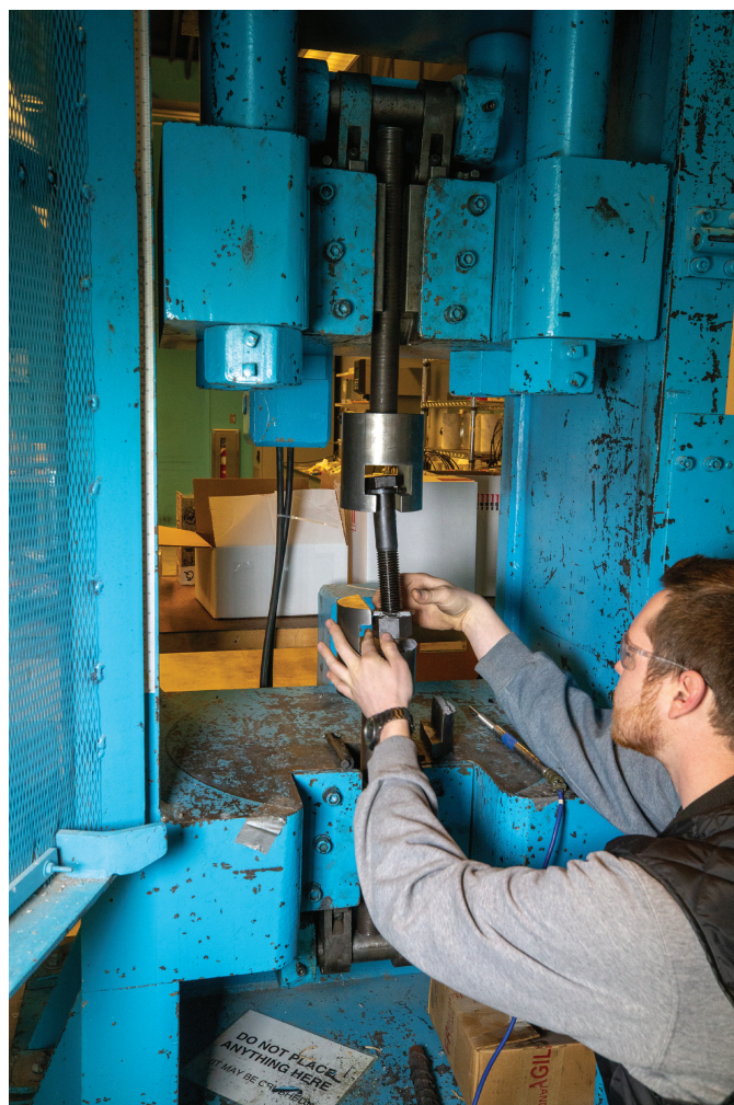
Fig. 4-1. Tension test (photo courtesy of Simpson Gumpertz & Heger).
