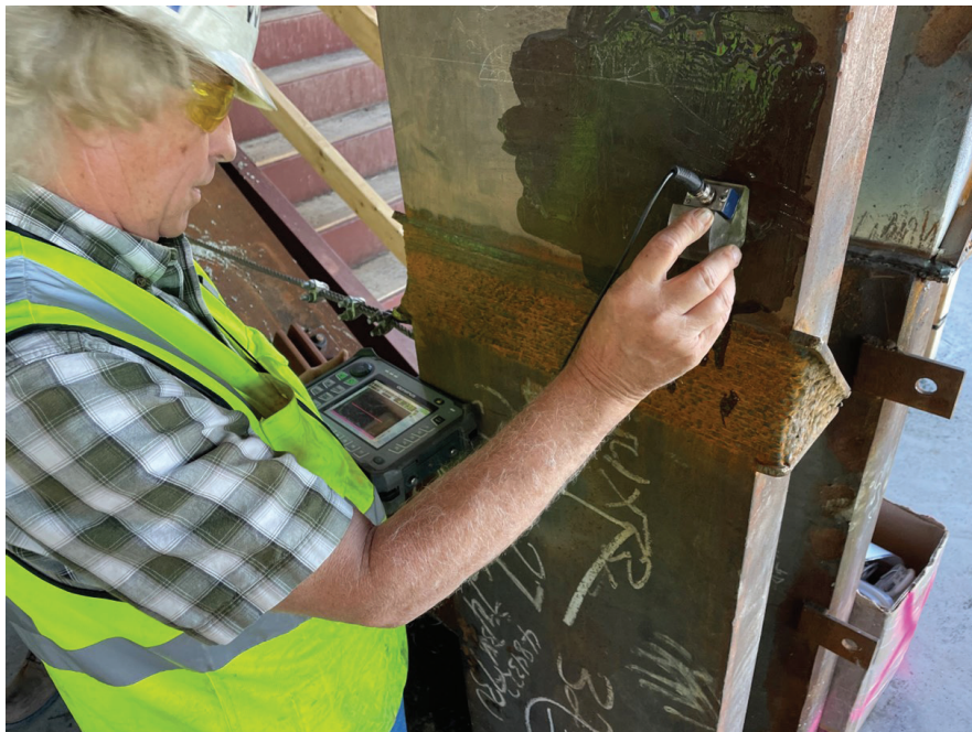
Fig. 3-8. Ultrasonic examination (photo courtesy of Simpson Gumpertz & Heger).
